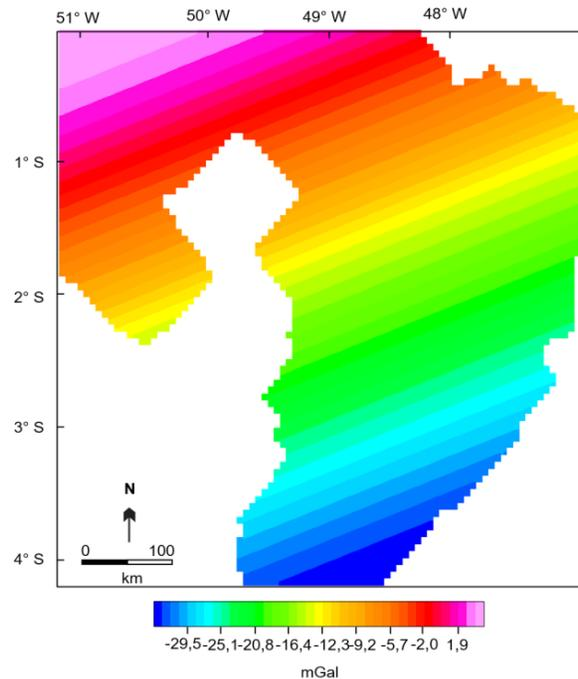
**Figure 4** - Map of gravity anomalies in the Marajó Basin for upward continuation of 32 km.
